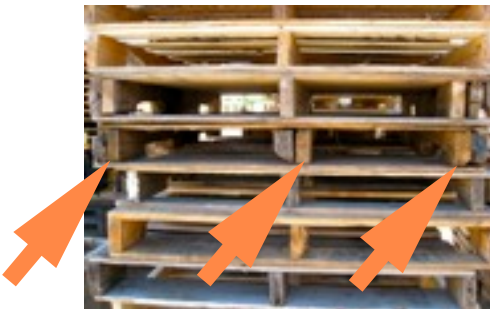
GMA TYPE 48" X 40" 09 A GMA style pallet, mixed wood species, with 7 top and 5 bottom deck boards (typically) and 4" or 6" lead boards. These pallets have block repairs on all stringers. They may have a broken runner as well as plates and corrugates. Stock# 4840-09
