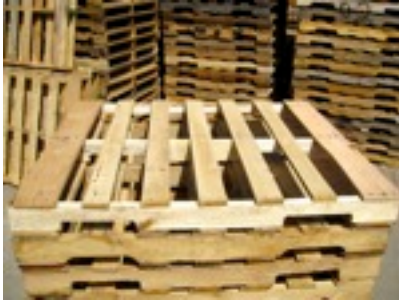
GMA 48" X 40" GRADE A PALLET 00 A GMA style pallet, mixed wood species, with 7 top and 5 bottom deck boards (typically) and 6" top and bottom lead boards (flush with the stringers). These pallets have no block repairs, plates, or corrugates. Stock# 4840-00
